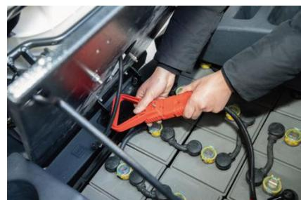
· The power system of this floor scrubber is composed of 16 2V lithium battery (or 6 piece of 6V no maintenance battery) charge in series, and the system voltage is 36V;
