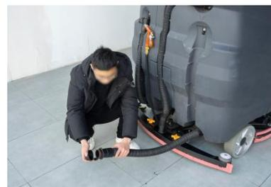
**⚠ Caution:** When flushing the recovery tank, do not splash water into the suction port to prevent the suction motor from burning out.
