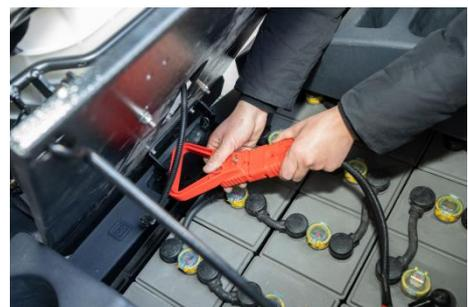
**⚠ Caution:** Due to the different distances of logistics routes, in order to avoid battery loss during long journeys, the battery cables have been disconnected at the factory.
