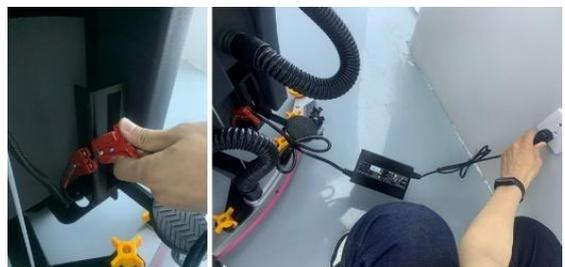
has undervoltage protection function, when the machine voltage is less than 21V, it will automatically cut off the power, and prohibit to use the equipment, then you need to charge in time, and continue to use.
