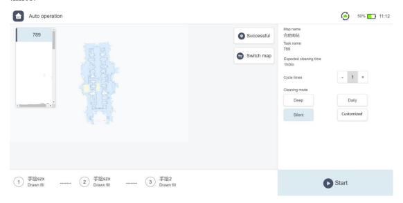
After completing the settings, click the [Start Task] button at the bottom right corner of the page. The floor scrubber will carry out the task automatically according to the selected task, the cleaning mode and the cleaning times. Operation steps are as follows:
